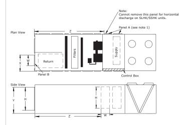
Custom Order Design (COD) now has a Design Special available to swap the location of the Control Box to the reverse side of the unit (right side) in order to allow supply airflow through the left hand (service access) side.
