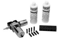
Flexible shaft repair kits include 4 drive end repair couplings, 4 thrust washers, 4 tool end repair couplings, 1 crimping tool with punch, 1 flexible shaft lubricator with quick disconnect, and 2 bottles (16 ounces) [0.5 liter] each of lubricant for flexible shaft lubricator.
