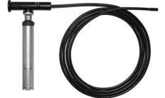
The FS-10 Tube Scope is ideal for inspecting the interior walls of boiler, chiller and condenser tubes. It can also be used to view the interior of ventilation shafts and ductwork, examine clogged drain lines, locate blockages in process pipes and identify hidden obstructions in walls. The unit comes equipped with a powerful battery powered halogen light, a flexible 10' (3m) fiber image probe with a 55 degree field of view, a 90 degree right angle view adapter and a durable carrying case.
