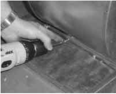
Step 7 Detach blower assembly from unit top panel.
