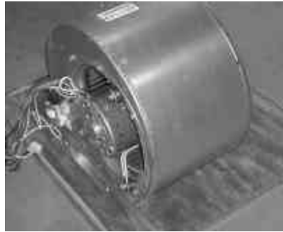
Step 8 Attach blower assembly to the back panel assembly. Note: Position the blower assembly to allow access to the motor through the side that is opposite end of the refrigerant-to-air coil.
