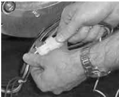
Step 10 Connect the motor via the 6-pin wire harness..
