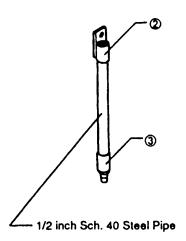
PIPE CUT LENGTH = Distance from Support Structure to top of heater less 4-7/8" (124 mm)
