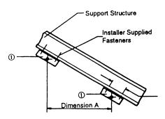
DIM. A = Distance between mounting holes.
