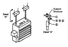
**Notes:** Connector (2) must be hung on the inside of Angle (1) as shown. Rotate connector to align with angle. Do not back off more than 3/4 turns.
