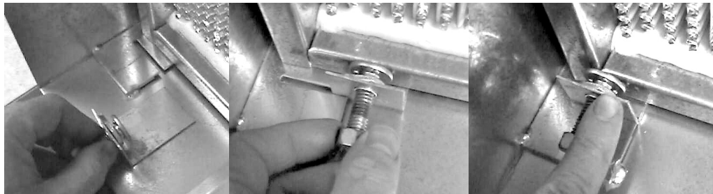
Figure 22. Tighten bolts with 9/16" socket or equivalent
