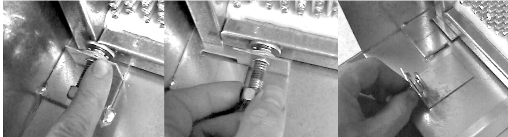
Figure 18. Remove the latch the bolt passes through
