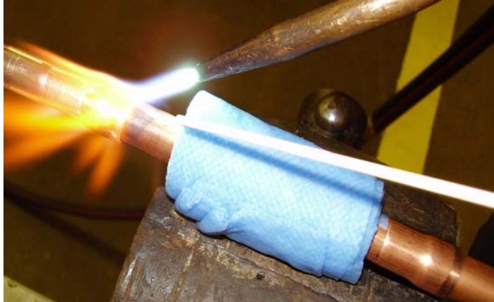
Figure 4. Direct heat away from components of part
