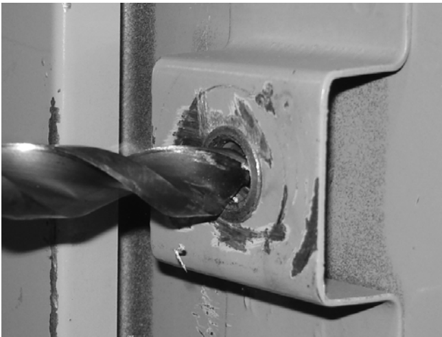
Figure 2. Drilling out rivet nut
