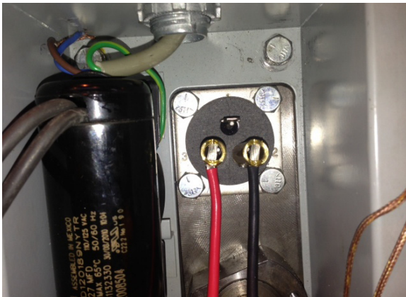
Figure 8. Installed Term-Lok adapter
