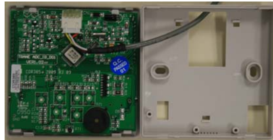
Cable through back cover and connected to circuit board
