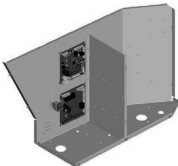
Figure 4. RTOM board mounted inside control box - method 2
