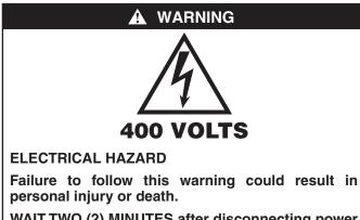
WAIT TWO (2) MINUTES after disconnecting power prior to touching electrical components as they may hold a dangerous charge of 400 VDC, then verify DC Voltage is less than 42 VDC at inverter test points labeled +VDC and -VDC before servicing board.
