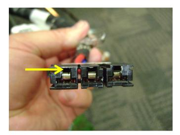
**Note:** If the connector plug is damaged when removing the terminals, discard the broken connector plug and use spare connector plug supplied with the kit.
