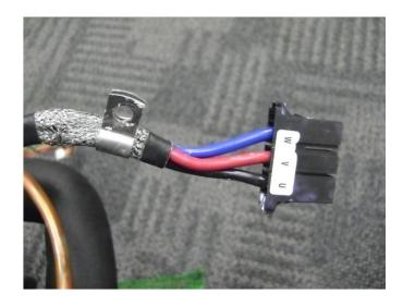
6. Using a paper clip or small screwdriver, insert 1/8" on top side of spade. Apply slight pressure downwards to lift and release the latch. Remove the terminal.
