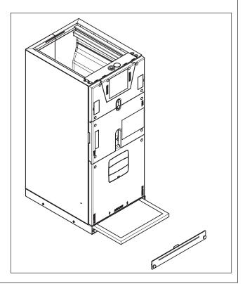
**Step 9** - Pictured is the finished filter box kit assembly. Continue the installation using the air handler Installer's Guide.
