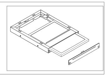
**NOTE:** A 2" filter cannot be used if also installing a BAYWMKIT001. This wall mount kit has a flange which will interfere with a 2" filter. The flange does not have an effect on the 1" filter.
