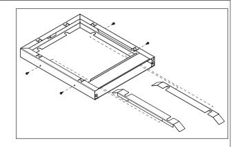
Apply the gasket material to create a seal between the air handler and the filter box
