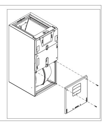
**Step 2** - Apply gasket material onto three sides of the bottom plate as shown. The gasket should be applied along the outside edge of the bottom plate. The three pieces along the notch should be applied so that the gasket material hangs off half the width of the gasket material.
