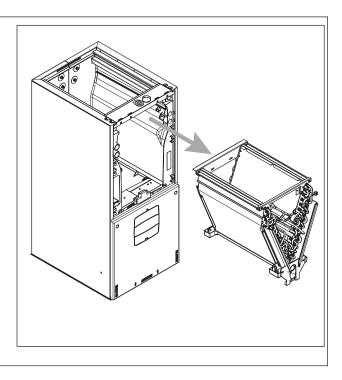
**Step 8** - Lift the air handler into place and set it onto the wall mount bracket.
