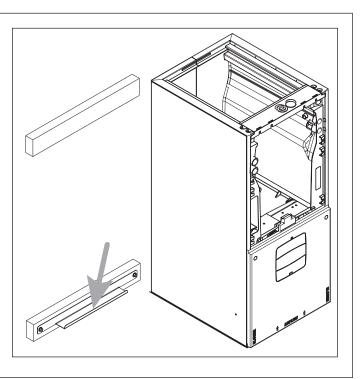
**NOTE**: Place a lock washer and flat washer onto the screws before attaching the cabinet to the mount material.
