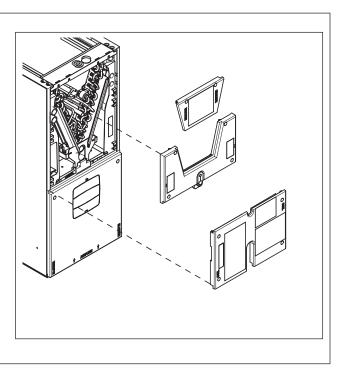
**Step 7** - Remove the coil from the air handler cabinet. See the air handler Installer's Guide, if needed.
