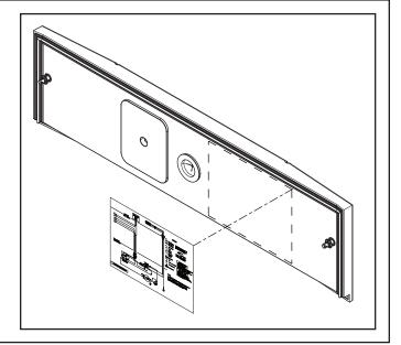
**STEP** 11 – Replace Heater compartment panel on air handler.
