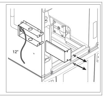
**Step 9** - Connect the wires to the low voltage terminal strip per the air handler Installer's Guide.
