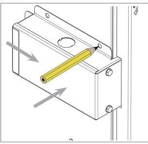
**Step 3** - With the entry kit removed from the air handler, remove the desired knock out.
