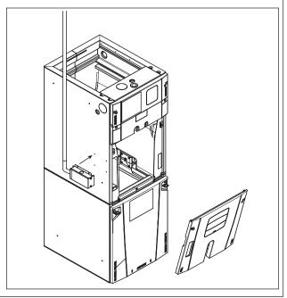
**Step 7** - Use the four provided screws to secure the conduit entry kit to the side of the air handler.
