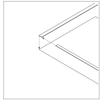
**STEP 5** - Attach the plate to the bottom of the air handler. Press firmly to make sure the double-sided tape adheres to the air handler.
