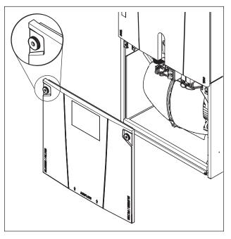
**STEP 4** - Remove the blower by first disconnecting the two wiring connections routed to the blower assembly.
