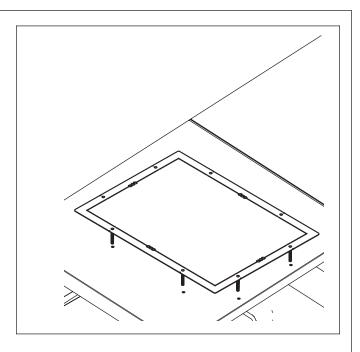
**STEP 11** - Place the template over the studs and secure with the nuts provided.
