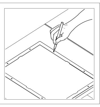
**STEP 9** - Use a 1/4 inch bit to drill each of the 8 points. The drill must be perpendicular to the air handler. The plate assembly will not fit through the holes if they are drilled in at an angle.
