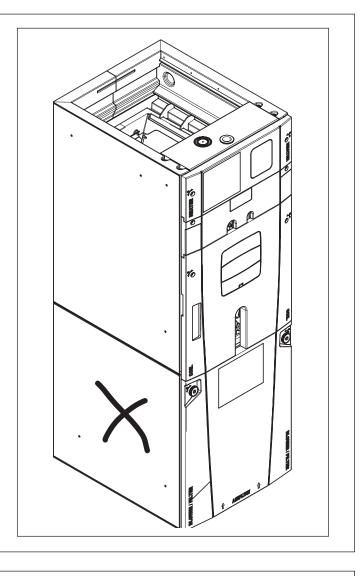
**STEP 3** - Remove blower panel once the proper side is noted.
