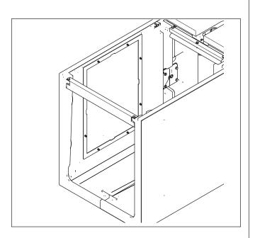
$\ensuremath{\mathbf{STEP~12}}$  - Drill out the three holes located on each side of the template
