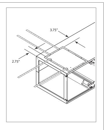
**Side Return Opening** - The inside dimension of the side return opening will be 11.0" x 15.5" If used, add 0.75" for the supplied flange.
