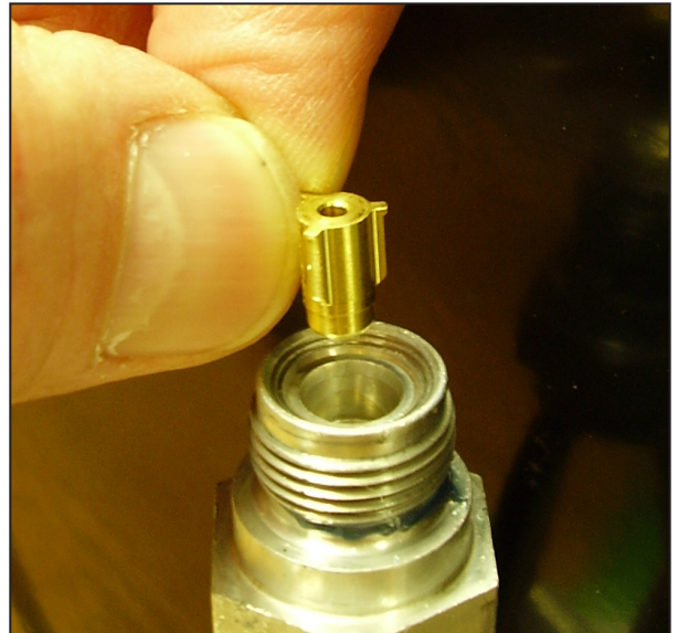
Figure 12 – Orientation of FCCV
