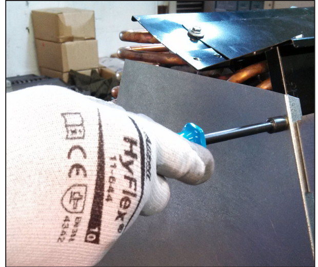
Figure 2 – Removing outer sheet metal cover
