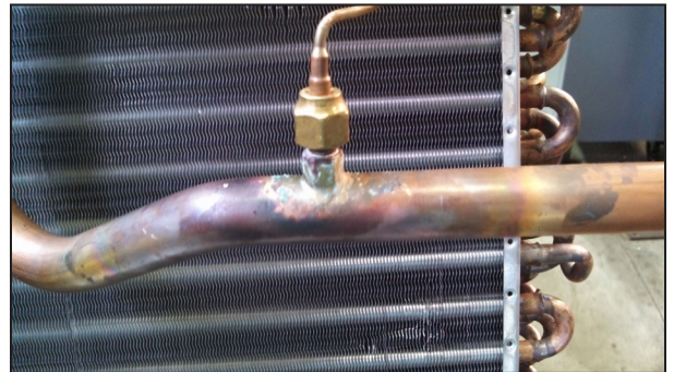
Figure 9 – Connecting equalizer line
