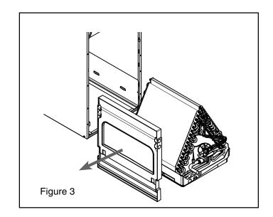
Remove screws from water diverter bracket. Make note of diverter position on the tube sheet (See Figure 4).
