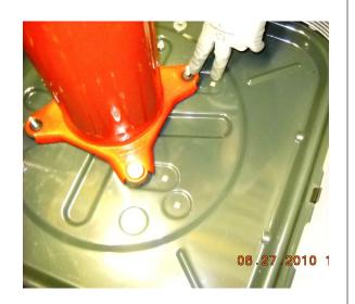
Using a ½" deep well socket remove the four nuts and washers from the compressor mounting bolts.
