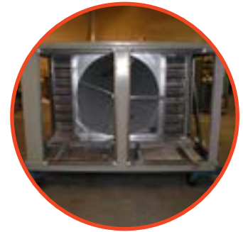
Internal Wheel with Economizer and Bypass Dampers
