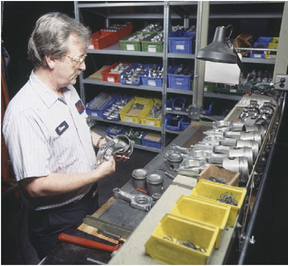
5. Subassembly: New or requalified parts are reassembled into rod and piston, valve cage, hand hole control covers, and oil pump subassemblies.
