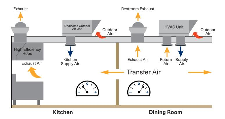
Here we see a properly balanced HVAC system, which uses an innovative Total Kitchen HVAC® design and includes a Trane TOAU. Make-up air units are not needed with this system. Positive pressure in the dining area keeps poor quality air out. Humidity and temperature are maintained at optimal levels. Energy costs are reduced. Guests and employees are more comfortable.
