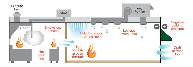
In this illustration we see the results of a poorly designed and improperly balanced restaurant HVAC system. Negative pressure in the dining area causes outside air to flow in through the front door, causing drafts and cold or hot spots. Air also flows in from the kitchen, bringing in odors, smoke and heat.
