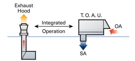
Total Kitchen Heating Ventilation and Air Conditioning\* (TKHVAC) is a system that uses high efficiency kitchen hoods with variable hood exhaust controls based on cooking loads. TKHVAC is integrated with Trane TOAU to replace kitchen hood exhaust with properly conditioned outside air. These measures increase restaurant energy efficiency by 20 to 35%.
