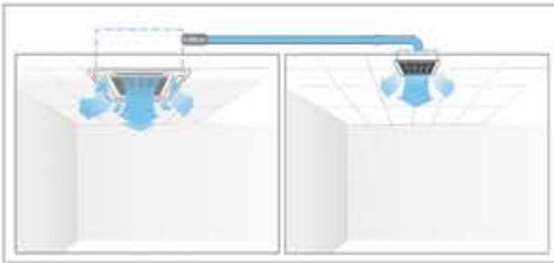
External air duct
