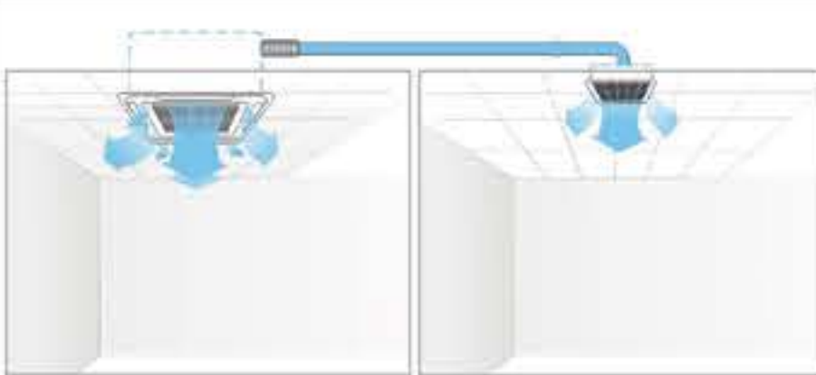
External air duct
