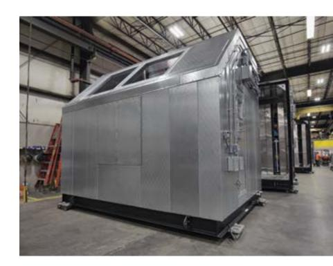
Casing options include galvanized steel, stainless steel or aluminum.
