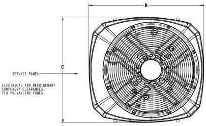
TOP DISCHARGE AREA SHOULD BE UNRESTRICTED FOR AT LEAST 1524 (5 FEET) ABOVE UNIT. UNIT SHOULD BE PLACED SO ROOF RUN-OFF WATER DOES NOT POUR DIRECTLY ON UNIT. AND SHOULD BE AT LEAST 305 (12") FROM WALL AND ALL SURROUNDING SHUBBERT ON TWO SIDES. OTHER TWO SIDES UNRESTRICTED.
