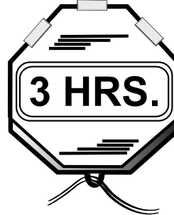
Figure 34. Wait at three hours before starting the unit
