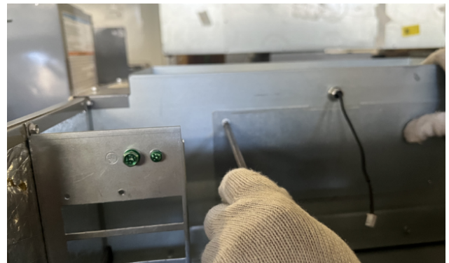
Figure 4. Disassemble metal plate
