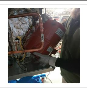
**STEP 3** - Prior to setting base plate, install pallet nuts, bolts and recip bushings onto the base plate. Secure base plate into compressor compartment.
