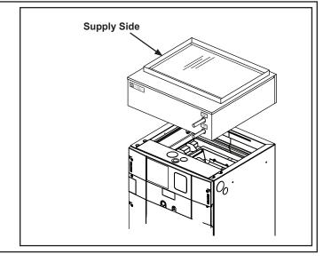
**STEP 3** - Wrap the coil attachment flange around the air handler and coil. It should have equal amounts of material covering the coil and air handler cabinet.
