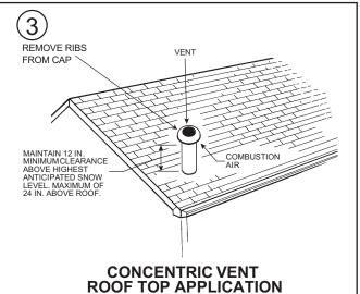
Remove ribs from rain cap. Install the rain cap and the small diameter pipe assembly in the Wye fitting and pipe assembly. Ensure that the small diameter pipe is cemented and bottomed into the Wye fitting.
