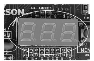
On a call for heat or cool, the display will continually alternate to indicate the mode and blower flow. If a fault occurs, the fault code will be additionally shown.
