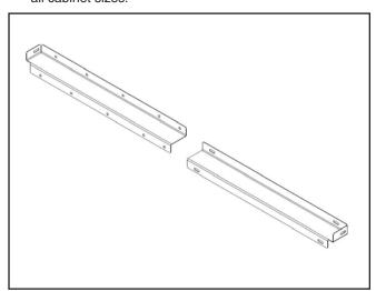
Using #8 screws, attach the blanking strip to the coil and furnace. Seal as needed and per local code to ensure an airtight fit.
