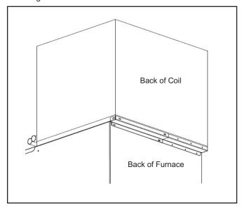
Combine the two sections in order to properly fit the appropriate cabinet size. The screw locations are shown as per figure below.
