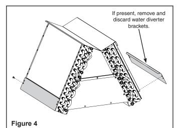
REQUIRED FOR HORIZONTAL LEFT COIL CONVERSION ONLY. Splash Guard installation is required to prevent water blowoff.
