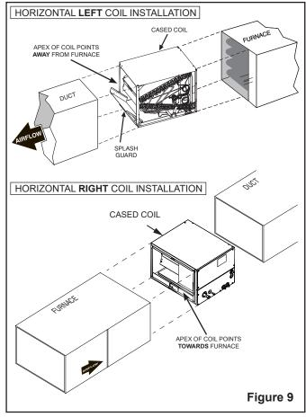
Attached furnace and coil using field-supplied self-drilling scews not longer than 1.5".
