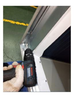
**STEP 5** - Reinstall the lower front panel using the screws removed in Step 1.
