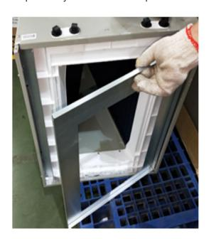
**STEP 4** - Align the back of the shield to the same height as the side channels and drill a 1/8" pilot hole through the side channel opening of the heat shield. Install one screw per side.
