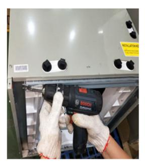
**STEP 3** - Place heat shield as shown with flanges down, and align the thru holes of the shield with the engagement holes of the coil support. Install the four screws previously removed from Step 2.
