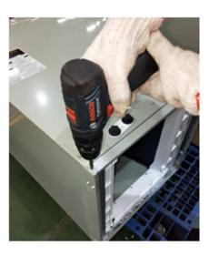
**STEP 2** - Remove the four 1/4" screws from the front channel. Retain the screws and discard the channel.
