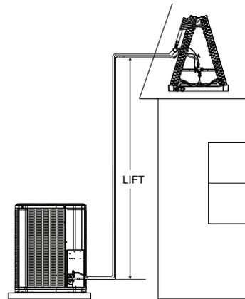
2. Determine the final subcooling value using total line length and lift measured in Step 1 and the tables below.
