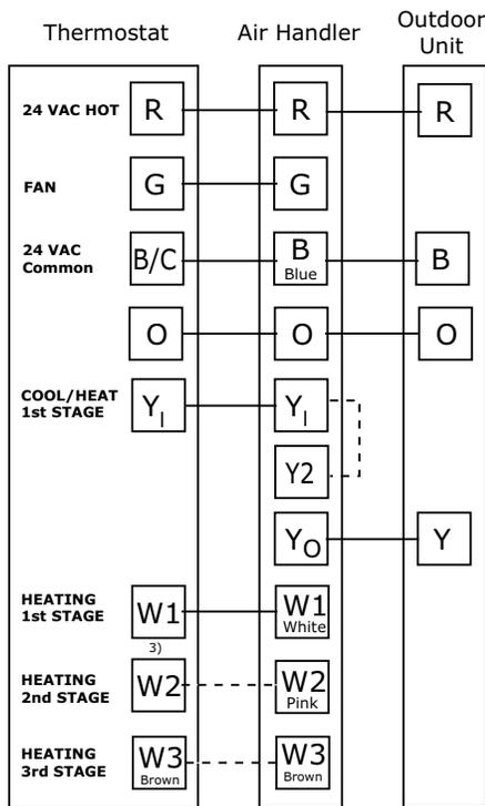
1. Units with pigtails require wirenuts for connections.
