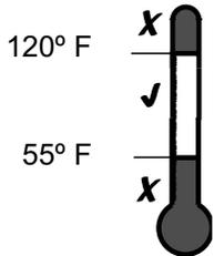
For outdoor temperatures below 55° F, See “Subcooling Charging Below 55° F Outdoor Temp. (In Heating Only),” p. 24.
