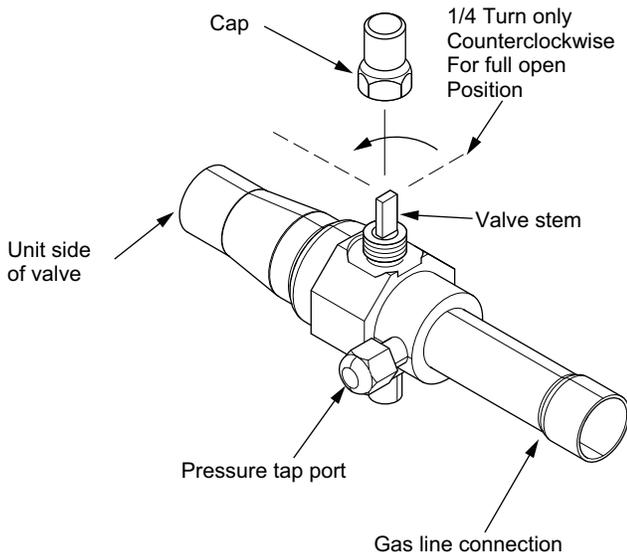
**Important:** Leak check and evacuation must be completed before opening the service valves.
