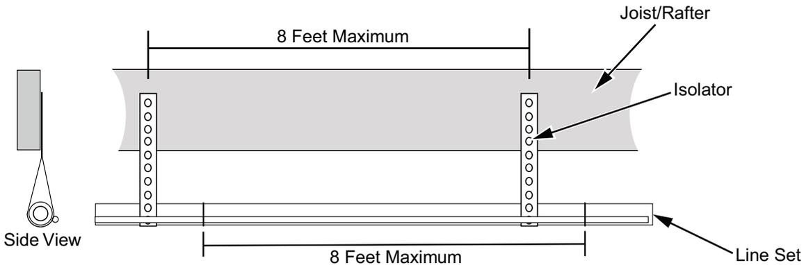
Secure the vapor line using isolators every 8 feet. Secure the liquid line directly to the vapor line using tape, wire, or other appropriate method every 8 feet.
