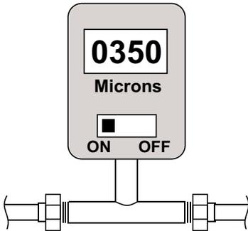
2. Observe the micron gauge. Evacuation is complete, if the micron gauge does not rise above 500 microns in 1 minute and 1500 microns in 10 minutes.
