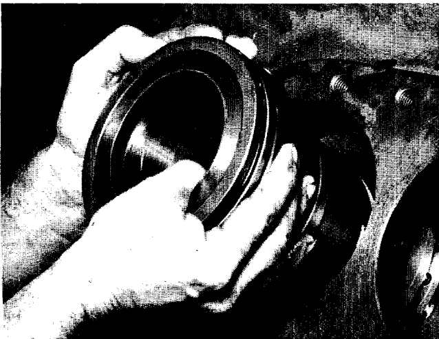
FIGURE 8—Pulling Cylinder Liner.
