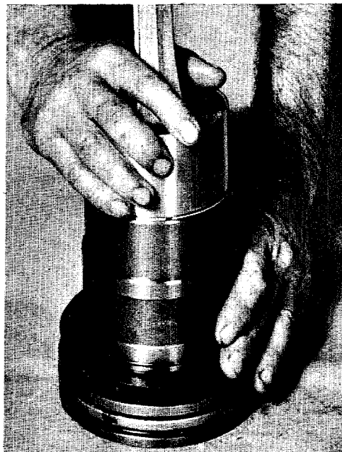
FIGURE 26—Inserting Piston and Connecting Rod Assembly Into Liner.
