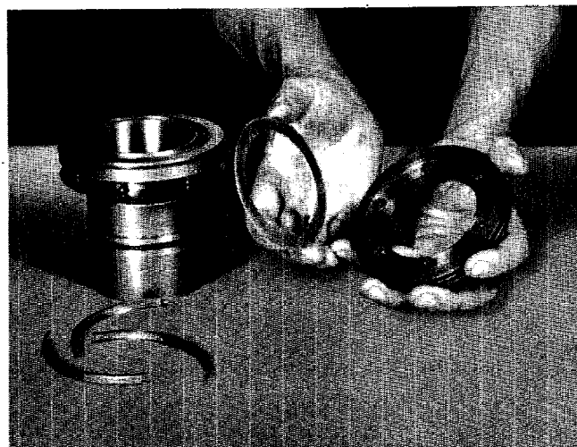
FIGURE 17—Removing Suction Valve Ring.
