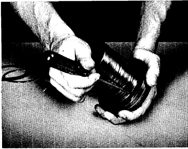
FIGURE 19—Checking Suction Valve Movement.
