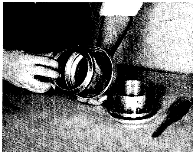
FIGURE 12—Removing Seal Ring.
