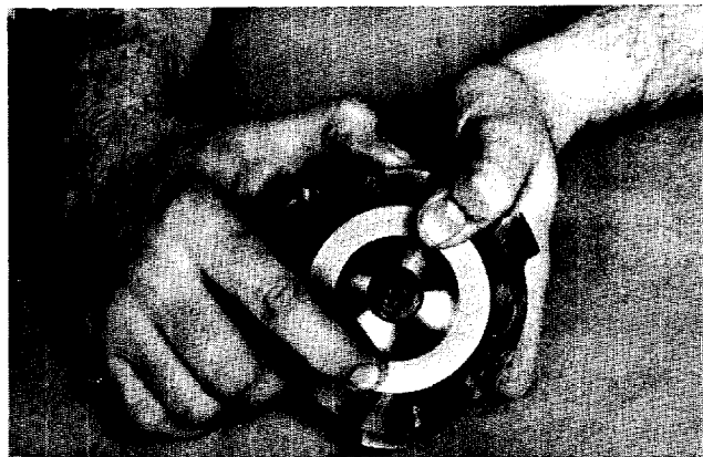
FIGURE 5—Checking Valve Movement.
