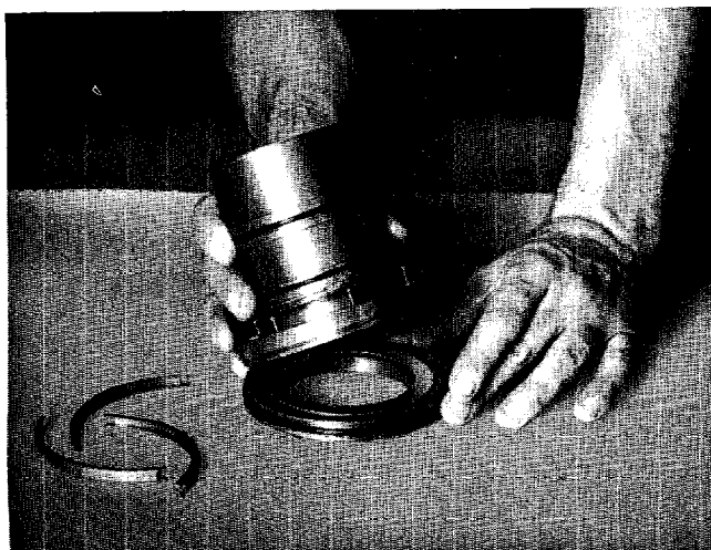
FIGURE 15—Lifting Off Liner.
