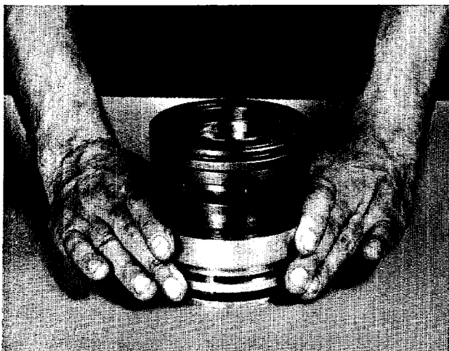
FIGURE 10—Removing Unloader From Liner.
