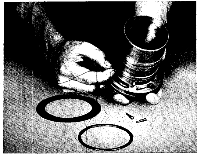
FIGURE 21—Inserting Springs and Lift Pins.
