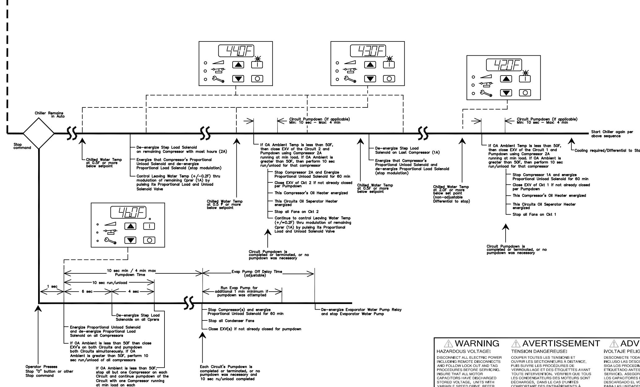
NOTE: This time line depicts a typical sequence of operation for a packaged RTAC Chiller with 4 compressors as it might perform with small pull down load, followed by a steadily increasing ramp load to greater than the rated chiller capacity, followed by a steadily decreasing load. The starts and hours of each compressor, used for determining lead-lag in this example, are as follows:
