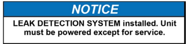
Figure 4. Proper labelling with leak detection systems is required on equipment. Image from: Understanding A2L Refrigerants and Changes to Governance in Air Handling Equipment CSAA/PSCA/UCCA & Refrigerant coils – Trane Commercial HVAC Help Center
