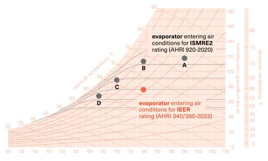
Standard 920 is intended to rate the dehumidification capacity and efficiency of a dedicated outdoor air unit, the evaporator must dehumidify the air to a target leaving-air dew point no higher than 55°F at test condition A. The leaving-air dew point at operating conditions B, C, and D must then be controlled to be within +/- 0.3°F of this target.
