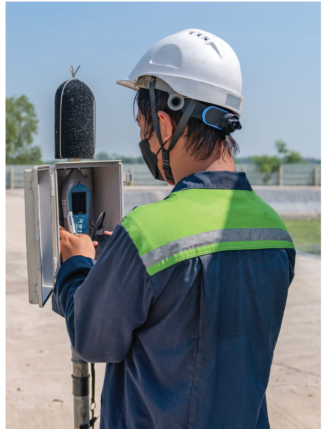
Environmental Officer Setting Sound Level Meter for Monitoring
