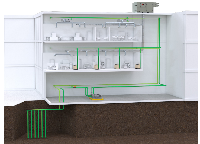
Distributed Geothermal System
