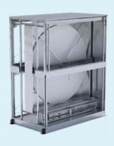
Air-to-air plate heat exchangers are a great solution to recover sensible energy (heat only) from an exhaust airstream, with little or no cross- contamination. These exchangers may also be used for free reheat in dehumidification applications, including dedicated outdoor air systems. Where exhaust air is not available, exchangers can be used in series to heat the dehumidified air.
