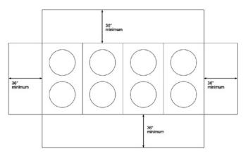
**NOTE:** If unit is surrounded by a fence, the minimum clearance is 48 inches. The fence must allow 50% airflow
