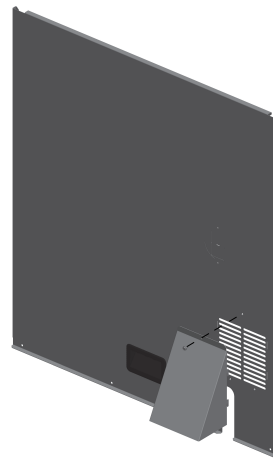
Figure 14. Vent hood installation
