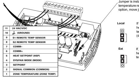
Jumper is installed from factory to display local temperature reading. To enable external sensor option, move jumper to **Ext** location.
