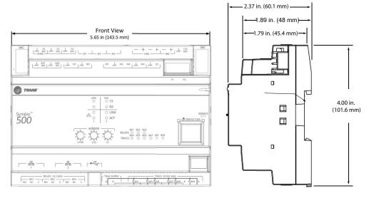
\*DIN Standard 43 880, Built-in Equipment for Electrical Installation. Overall Dimensions and Related Mounting Dimensions.
