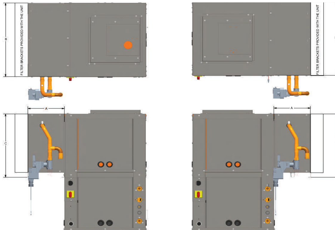
Figure 31. Waterside economizer (EXVK/DXVK)
