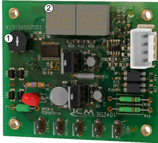
Figure 12. ECM control board
